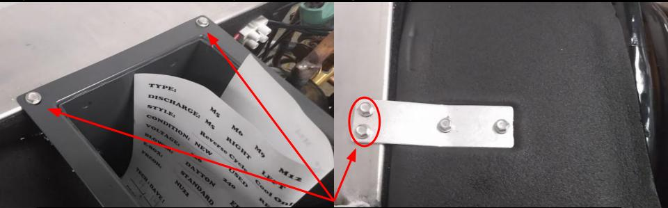
Temporarily remove these screws so blower can be separated from the shroud.
